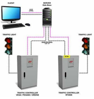
Traffic controllers and Clients must be able to communicate with the Central Server. Therefore, they must be under the same Central Server subnetwork or be equipped with an Internet connection.
