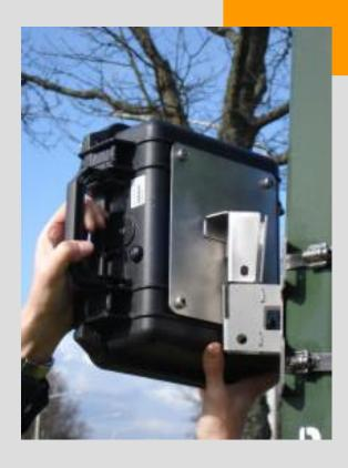
The TMS-SA is an above ground and portable traffic counter.
